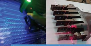
Generator parts 3D scanning and deformation inspectio
